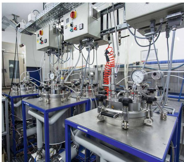
In these autoclaves, samples are exposed to excess oxygen and "cooked" at high pressure until they become brittle.
