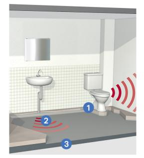
1) Because the installation elements for sanitary installations come into direct contact with the floor or the walls, sound is transmitted to the entire building.
