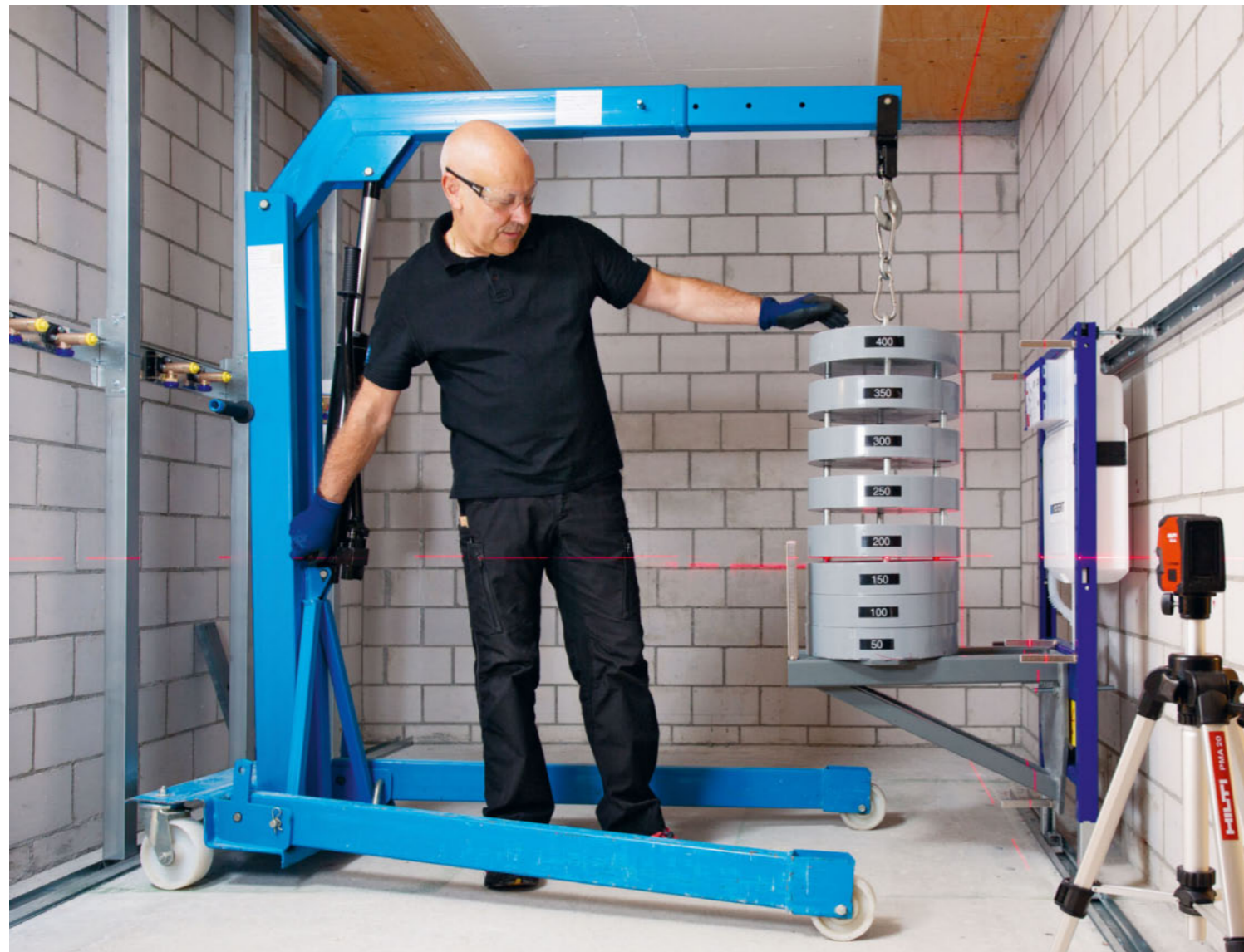
↑ One by one, Geberit statics specialist René Gmür carefully lowers the 50-kg-weight plates onto the special frame that is attached to a Geberit Duofix element.
