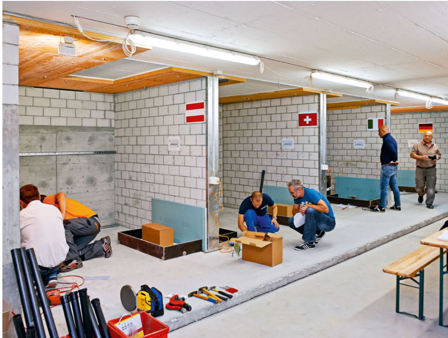
↑ Plumbers and tilers from four different countries install prototypes of the new Geberit shower channel CleanLine at Geberit's building technology and acoustics laboratory.
