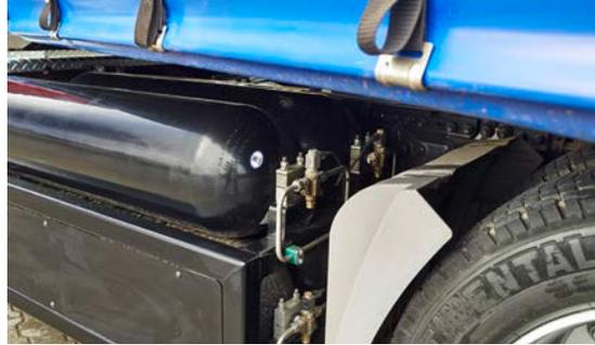
The eight natural gas tanks have a capacity of 640 liters. Fully tanked, the vehicle can travel a total of around 550 kilometers before it's time for a refill.
