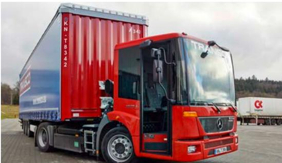
The driver's cabin of the natural gas truck is different to that of conventional diesel trucks, with the overall appearance and entrance reminiscent of a bus.
