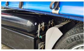
The eight natural gas tanks have a capacity of 640 liters. Fully tanked, the vehicle can travel a total of around 550 kilometers before it's time for a refill.
