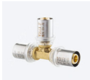
↑ The transparent plastic rings on the Volex press fittings make it easy to check the correct insertion depth.
